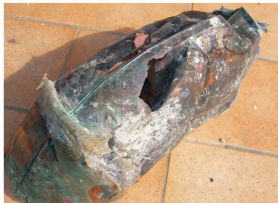
Fig. 3 - A metal pipe union of the water-rain drainage system of a terrace with holes and cracks (Photo by Renato D'Apuzzo)
