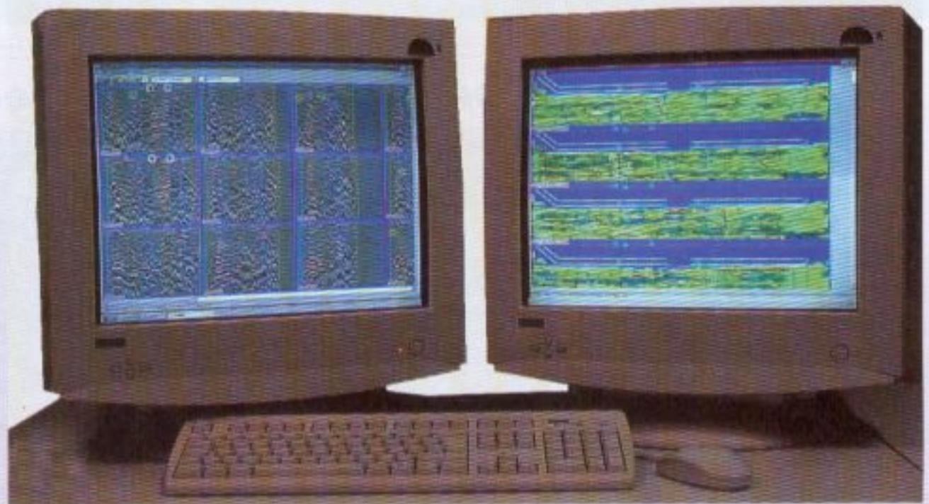
Using the RIS/MF system, an operator can view both the radar image (left) and a tomographic view.
