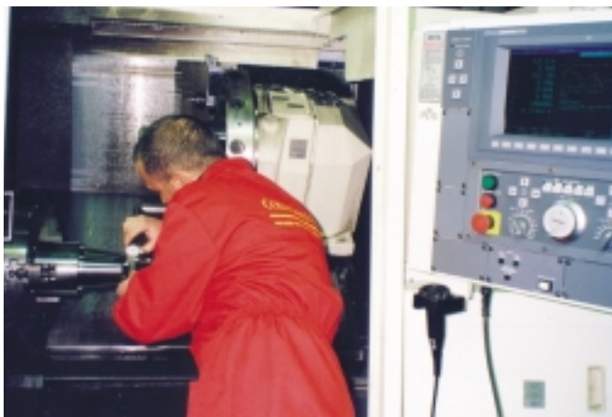
Finishing drill rod threads on a CNC lathe.
